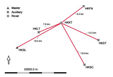
**Figure 12.** Distribution of auxiliary reference stations in relation to the rover station HKKT. Station HKSL was the designated master reference station.
