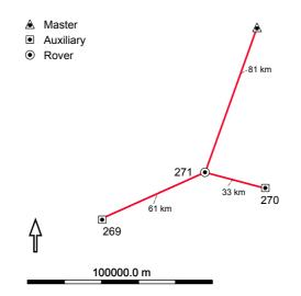
Figure 3 Distribution of reference stations in the test network. Station 258 was the designated master and station 271 was used to simulate the rover.
