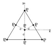
**Figure 1.** Hypothetical network of 6 reference stations and one rover station located at the centroid of the figure.
