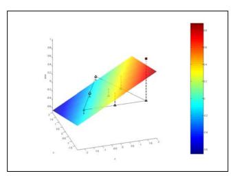
**Figure 2.** Case 1: the approximated error at a station P = (x, y) resulting from a bias at one of the reference stations  $P_1$ ,  $P_3$  or  $P_5$ .
